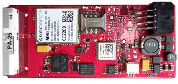
The KCS GPRS/GPS range of modules enables you to remotely track & trace people, animals and a variety of objects, e.g. cars, trucks, containers, (motor)cycles, lawnmowers, boats, etc.
