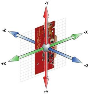
The module contains an optional 3D accelerometer (up to 16g), which can be used for a variety of custom specific (M2M) applications. Accelerometers are useful for measuring movement, speed, g-forces and vibration of the object. The accelerometer and advanced embedded firmware enables a very low-power battery solution.
